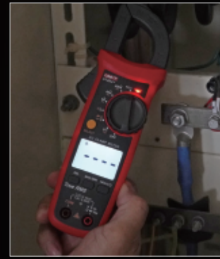
NCV multi-segment display and audio/visual alarm
