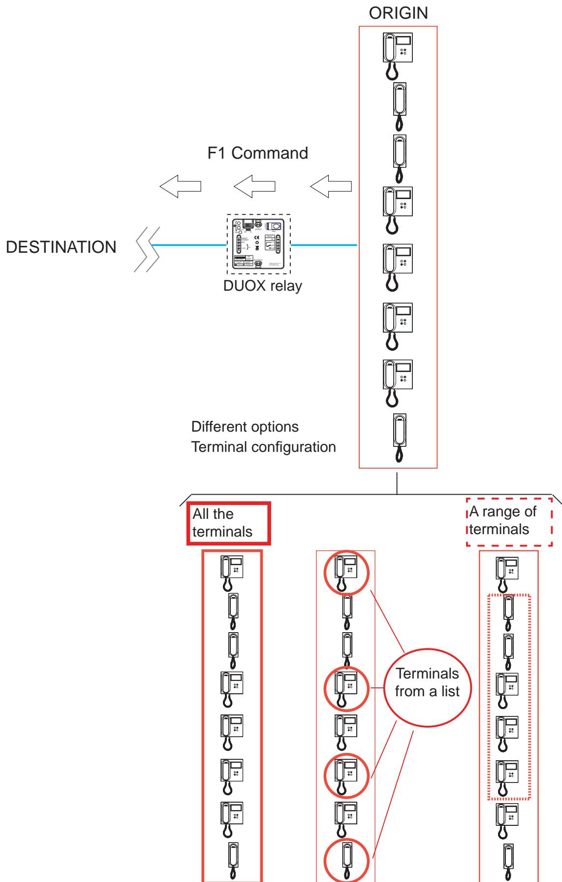
**Function configuration.****First step: Configuration of commands.**
