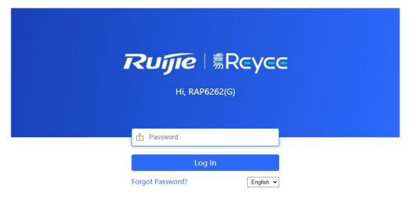
Username and password are not required at your first login and you can configure the access point directly. For device security, you are advised to set the management password after your first login to the web management system. After the password is set, you need to enter the password when you log in to the web management system again.
