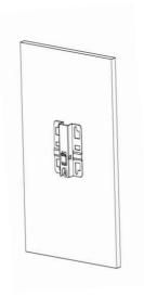
b Install the access point and the connecting rod to the mounting plate on the wall, and tighten the M8 x 20 screws to complete installation.
