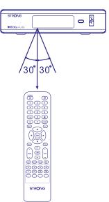
To use the remote control, point it towards the front of the digital receiver. The remote control has a range of up to 7 metres from the receiver, if properly aligned towards the IR eye on the front panel. The remote control will not operate if its path is blocked.
