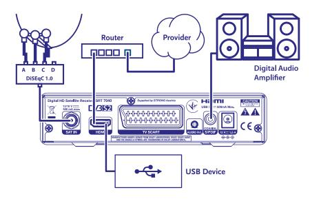
Connect one end of a good quality coaxial audio cable to the S/PDIF output of your receiver and the other end to the coaxial audio input of your home theatre, amplifier or any other device supporting digital audio.
